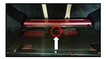
5. Take the rubber cap off and put the wires through at the outside length of approx. 60cm
