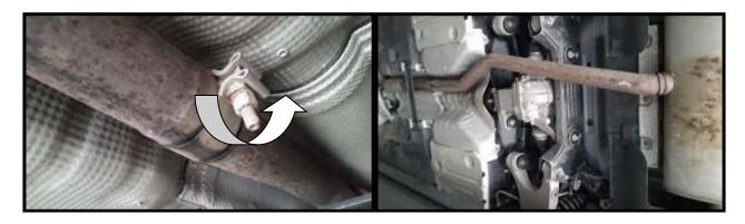
**3.** Connect the electric valve Place the central unit in the trunk of the car
