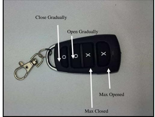
RC buttons explained (from the bottom) X – MAX Opened X – MAX Closed O – Open gradually O – Close gradually
