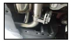
9. Test the RC operation – pressing the button should trigger the electric valve.
